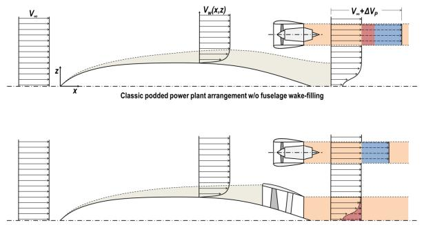
Propulsive fuselage device applied to ideal fuselage wake-filling only, required residual aircraft thrust provided by podded power plants
