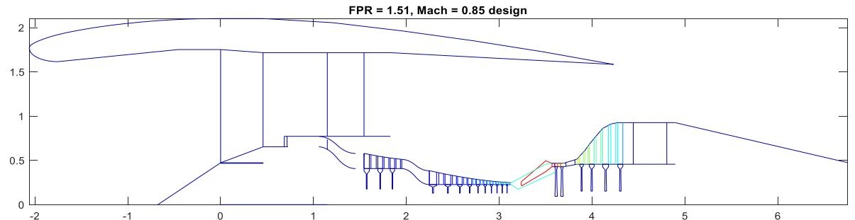
$$SFC_{installed} = \frac{b}{F_{Net} - D_{engine\ mass} - D_{nacelle}}$$
