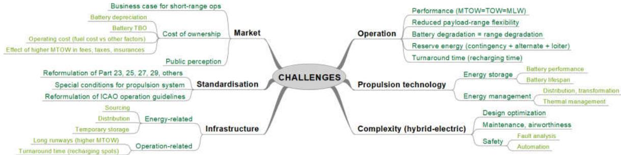
Figure 2. Some of the identified challenges for electric-powered commercial flight.
