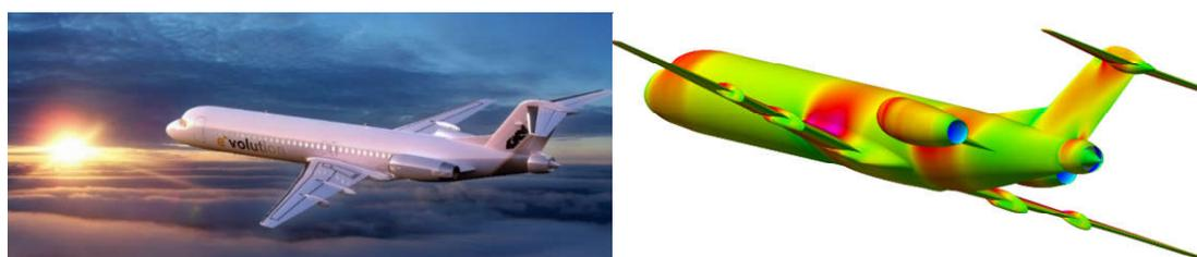
**Figure 1.** Artists view of the F100 TCT configuration and CFD result pressure distribution
