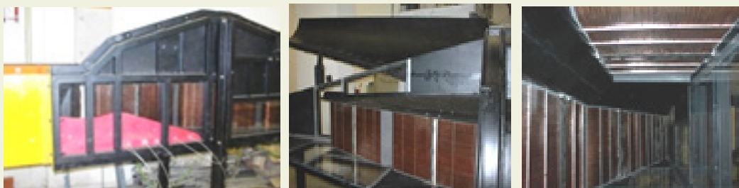
Figure 3. Reference nozzle configuration (AEROHEX) test-rig – 1/4 nozzle representation
