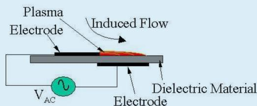
Figure 1. DBD plasma actuator configuration, figure from (Suzen et al. 2005).
