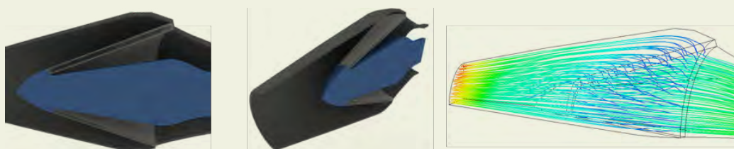
Figure 4. CORN (COncal Recuperative Nozzle) geometry and velocity streamlines.
