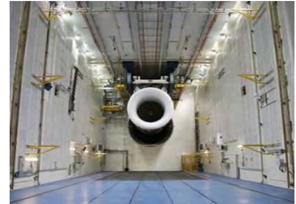
ALECSYS (Trent engine) System Commissioning
