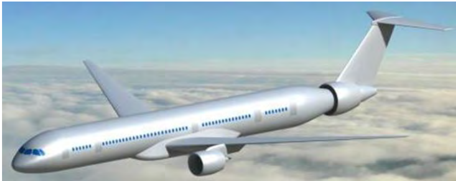
Propulsive-Fuselage Concept (PFC)
