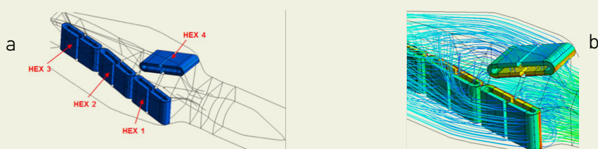
Figure 3a. NEWAC nozzle configuration, 3b. Swirl effects in NEWAC nozzle.
